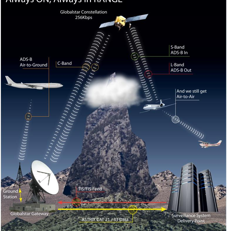
alcas is a true over-the-horizon air traffic management system capable of delivering an uncorrupted 1090ES or UAT payload from virtually any ADS-B avionics system to a Surveillance System Delivery Point (SDP) in near real-time from oceanic, remote or mountainous areas where a conventional line-of-sight connection to a terrestrial ADS-B ground station is either impossible, or impractical. The target cost for ADS-B reports should be less than current ADS-C services.
